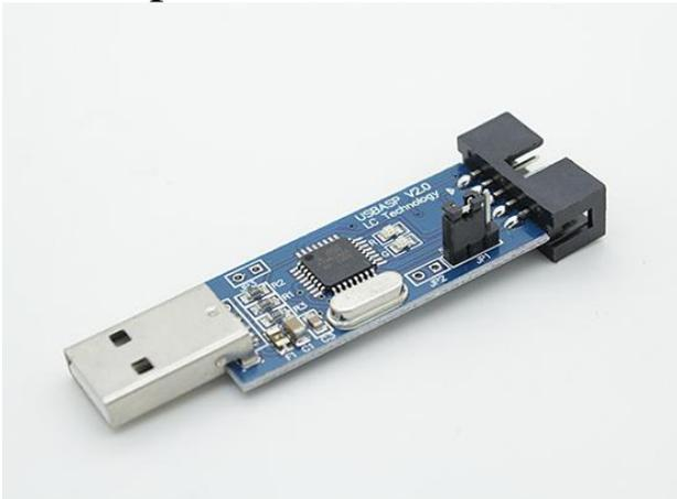
The most convenient adapter to go with the above socket tool, is the USBasp.
